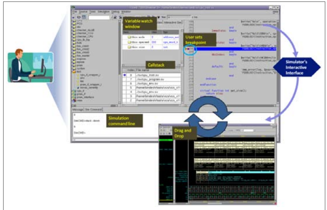
Figure 2: The use of a unified and full-featured debug system to drive interactive testbench simulation can allow for more user-friendly set-up and visualization and analysis of results.
